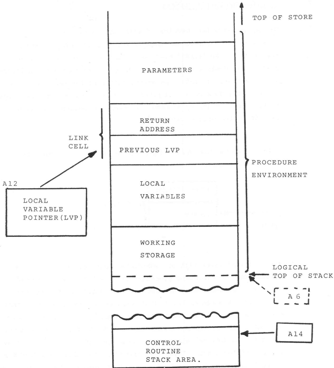
Fig. 2.1. - STACK LAYOUT OF A SINGLE PROC.
