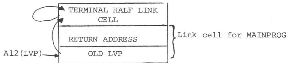
2.3.4. Currently, all run-time support packages have start-up routines which use this convention. They are independent of the characteristics of the user's programs which must always be entered by a procedure of the same name. Every user's main program would therefore have the following RTL/2 specification:
