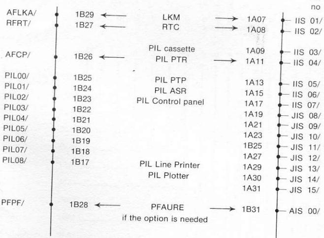
signals into connector of card OPTI
